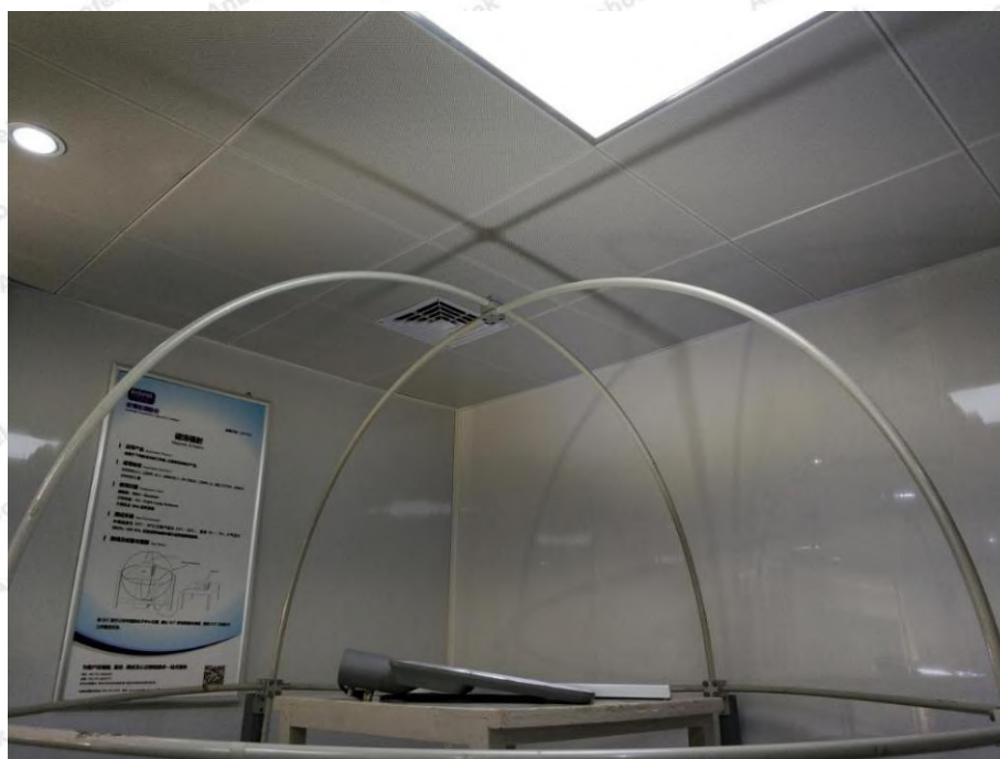
Photo of Magnetic Radiated Emission Test
